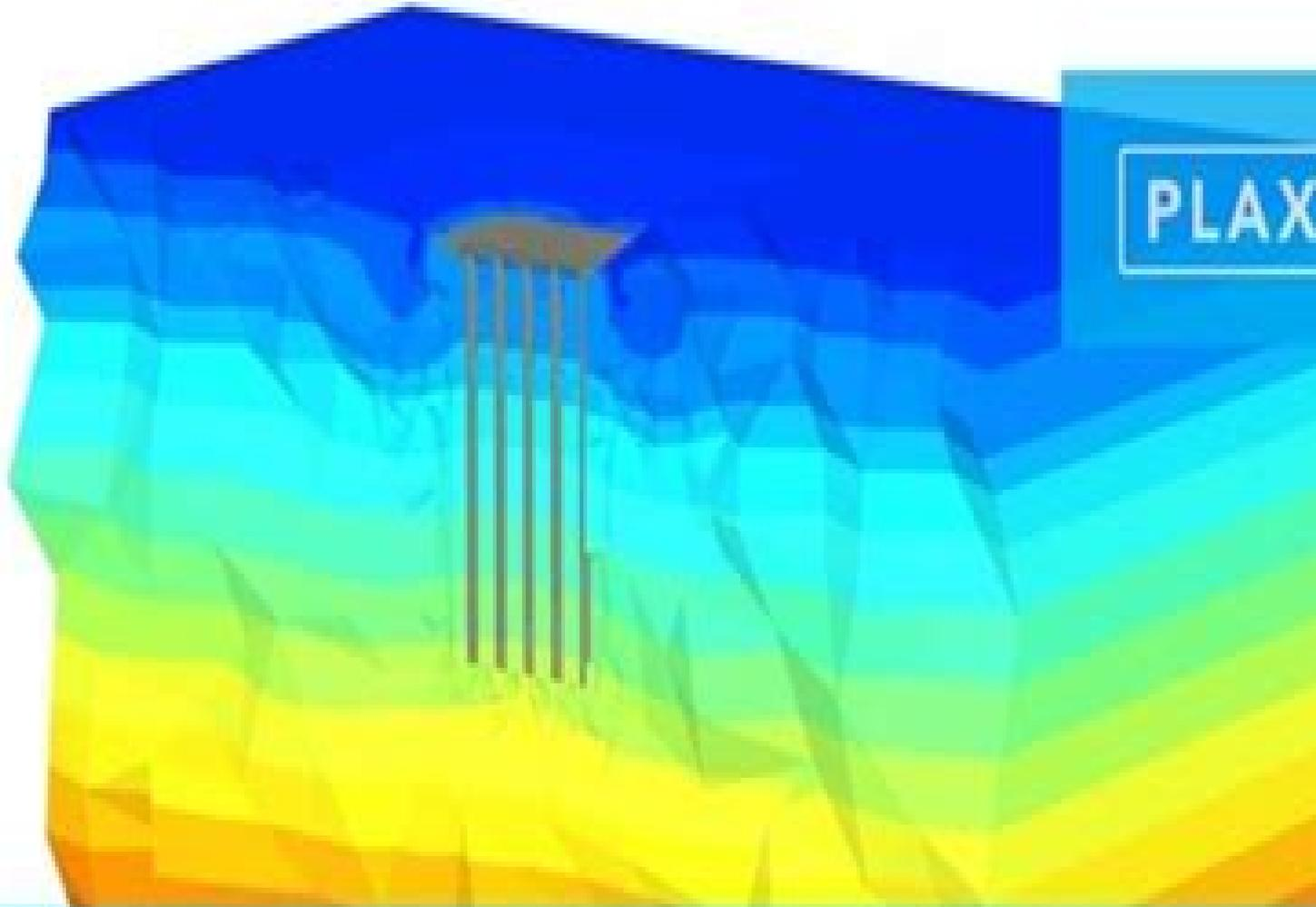
A 3D finite element model of a pile group in soil. The soil is represented by a mesh of elements, colored with a vertical gradient from blue at the top to red at the bottom. Five vertical piles are shown, connected by a horizontal cap. The model is set within a rectangular domain. A blue box in the top right corner contains the text 'PLAXIS'.
