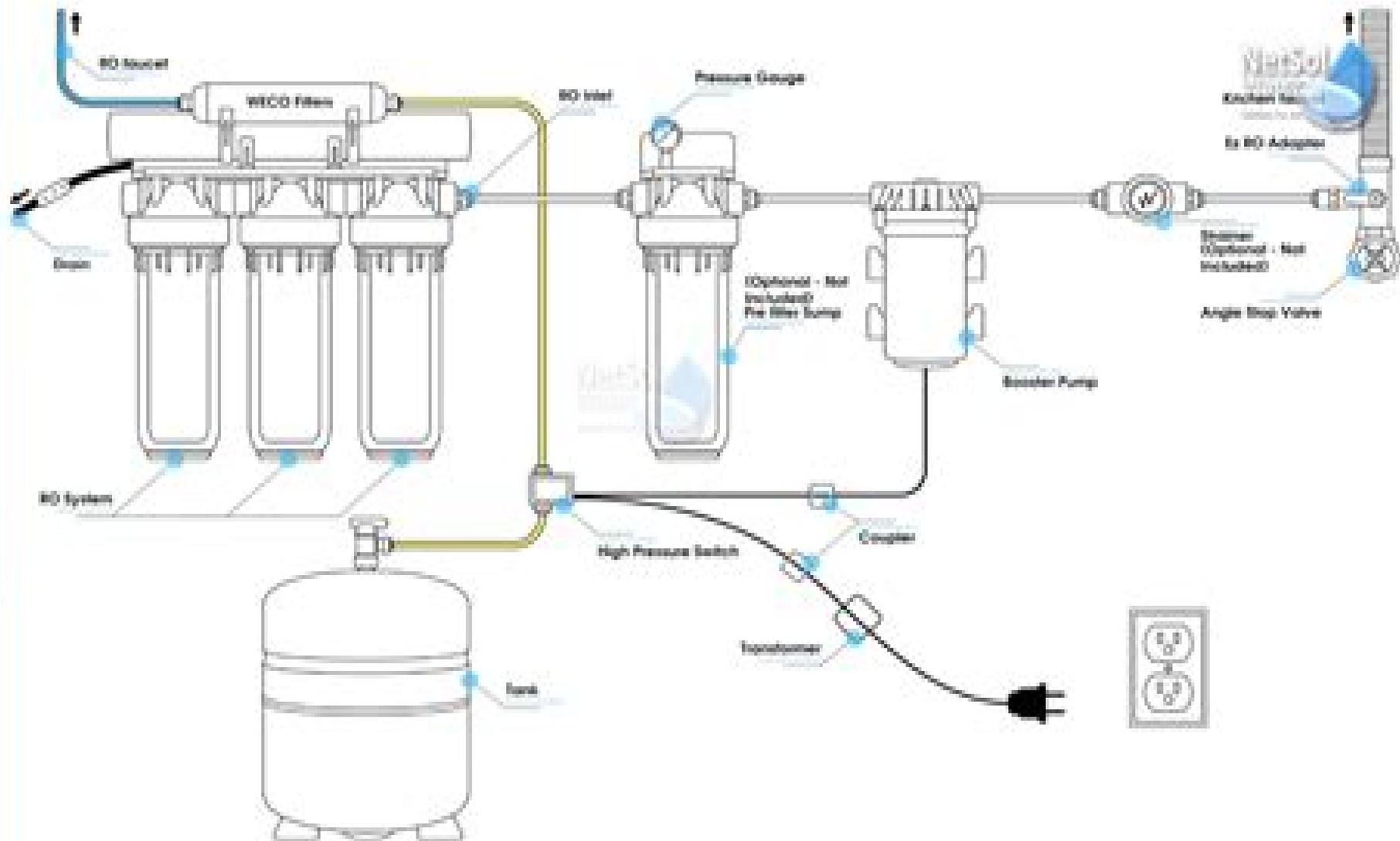
Schematic Diagram of Reverse Osmosis Plant With RO Components
