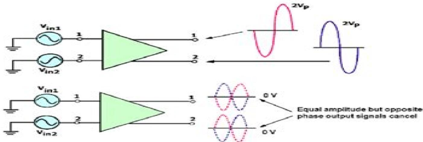
Figure 11.1: Differential amplifier shows differential inputs and common-mode inputs
