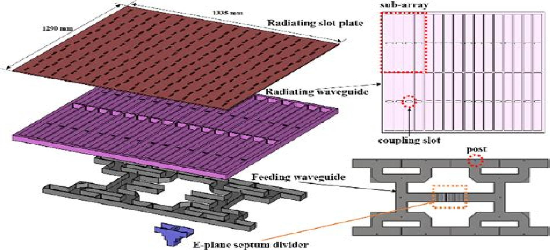
Fig. 1. Designed 16×16 slotted waveguide array antenna structures
