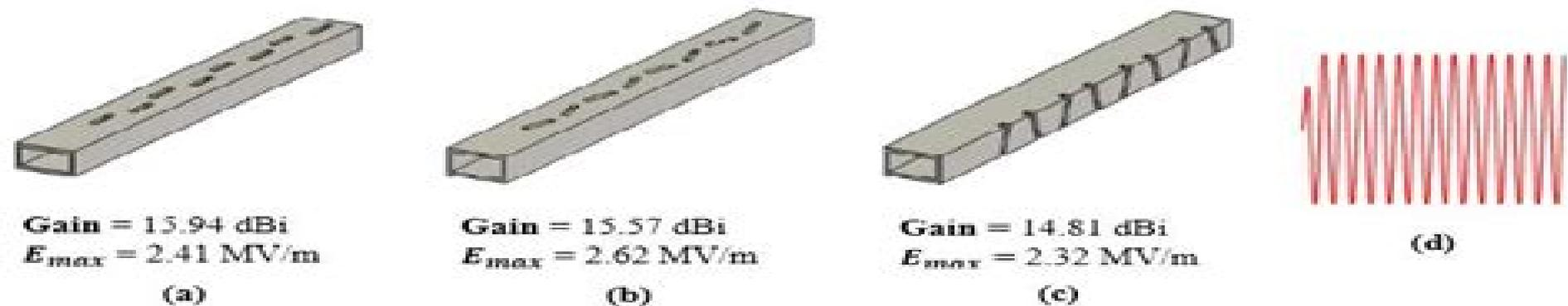
Fig. 2. Gain and maximum E field results (a) 8×1 longitudinal linear slot
