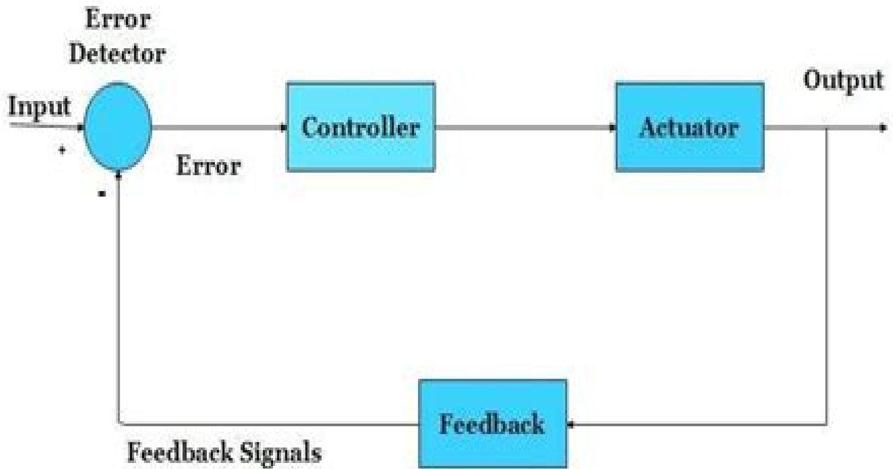
**Block Diagram for Process Control System**
