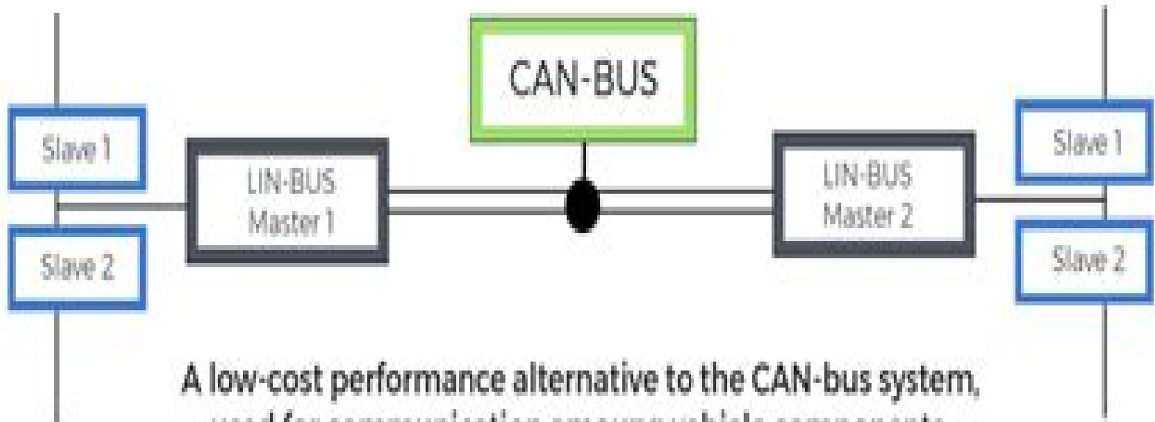
A low-cost performance alternative to the CAN-bus system, used for communication among vehicle components.
